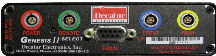
Figure 3b The Genesis II Select™ rear interface
